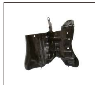
REINFORCEMENT FRAME BRACKET 911.TY44326A R:
