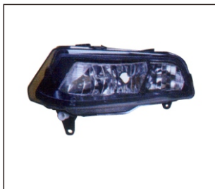
FOG LAMP ONE BULB HOLE 939.VWC331 R:6ED941662 L:6RD941661
