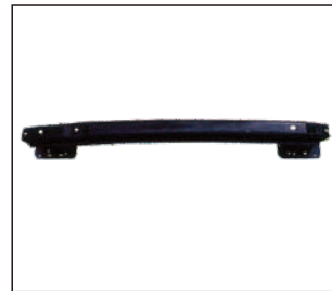
REAR BUMPER REINFORCEMENT 911.FD44023A OE:3M51403226AJ
