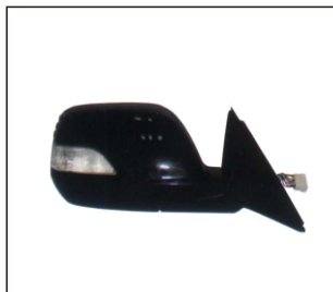
MIRROR ELECT,HEATED,FOLDABLE W/LAMP W/SENSOR 980.HD7125E R:76200-TZ8-H11 L:76250-TZ8-H11
