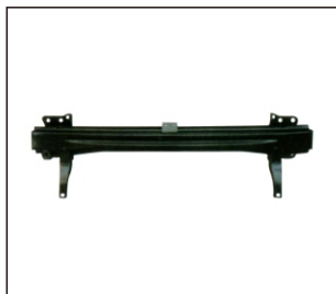
FRONT BUMPER REINFORCEMENT 911.6344323A OE:1K8807109B
