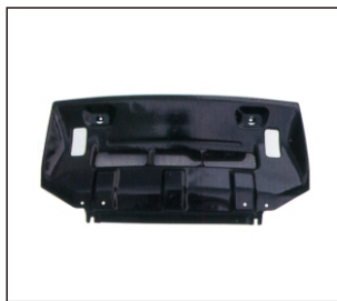
COVER, ENGINE UNDERBOARD 957.MB22015A OE:
