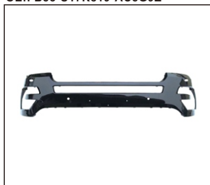
FRONT BUMPER W/SENSOR& WASHER HOLE 901.FD05038BA W/ TOW COVER 901.FD05038BB W/O TOW COVER
